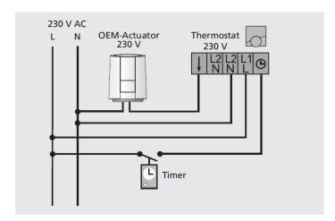
We recommend the following lines for installing a 230 V system:
