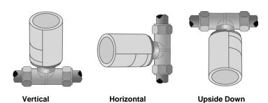
Preferred installation positions of the OEM-Acutator are vertical and horizontal. An upside down position may reduce product life through special circumstances (e.g. contaminated water).
