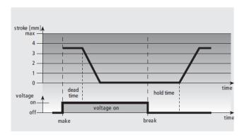
In case of the normally open version, the valve is closed evenly by the ram motion upon switching on the operating voltage and after expiry of the dead time.
