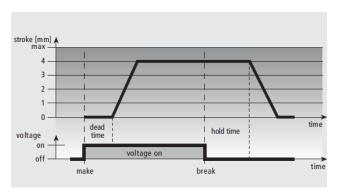
In case of the normally closed version, the valve is opened steadily by the ram motion upon switching on the operating voltage and after expiry of the dead time.
